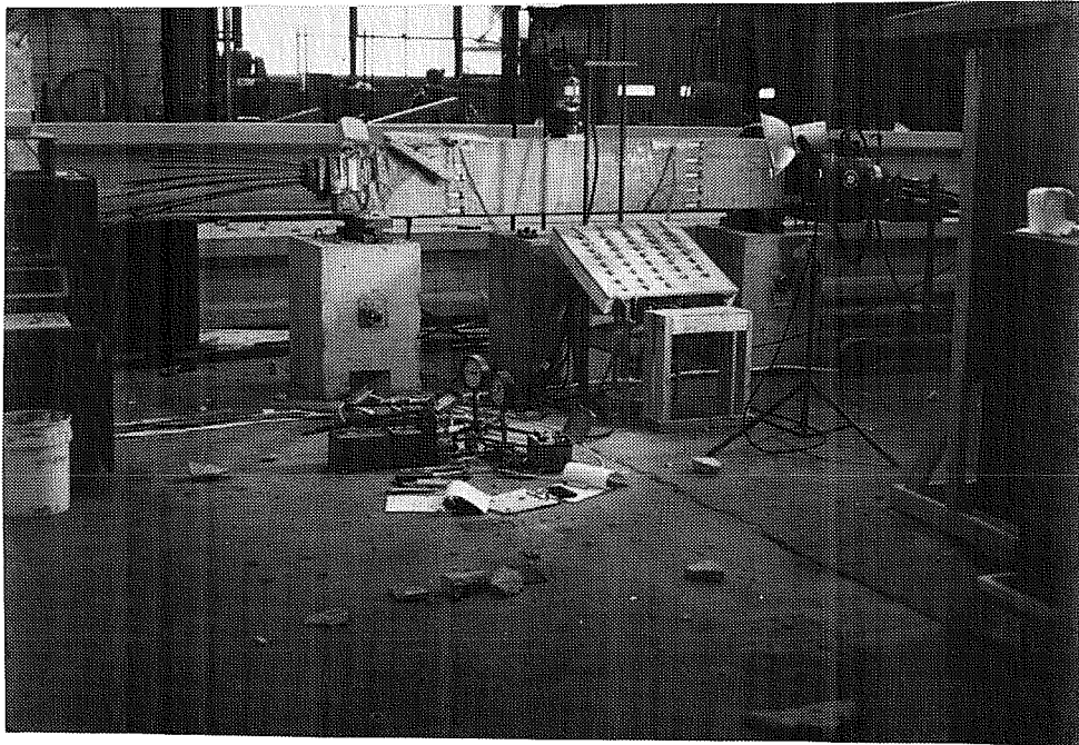
Figure 3.35 Explosive Failure of Specimen Beam2
