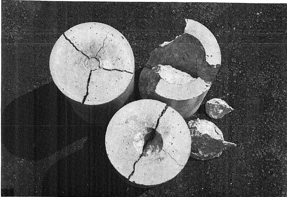
Figure 6.3 Splitting Failure of Cylinder Specimens with Various A/A_b Ratios
