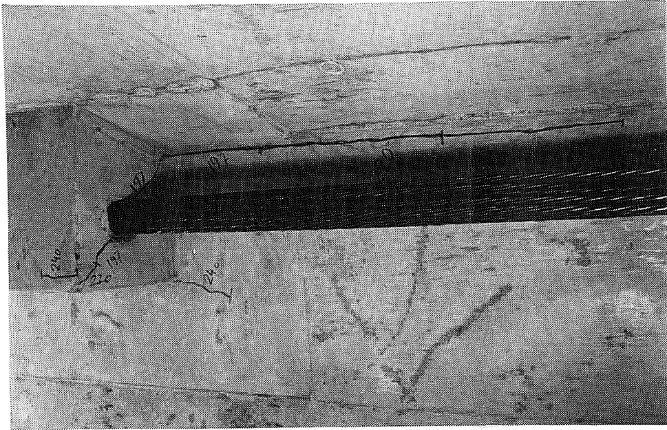
Figure 4.73 Crack Development In Specimen Corner3 at 94% of Failure Load
